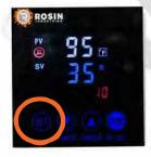
After desired time is selected, Press SET button twice to confirm time and return to main screen
