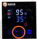
Press arrows "up" of "down" to select temperature as required
