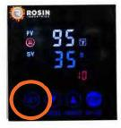
After desired temperature is selected, Press the SET button to confirm the setting
