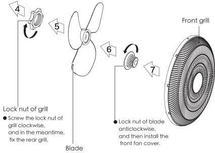
Pull the blade to rotate after installing, so as to ensure that the blade can be normally rotated.
