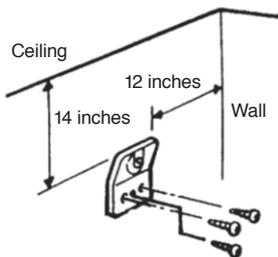
**NOTE:** The bracket should be positioned at least 14 inches from the ceiling and at least 12 inches from adjoining wall.
