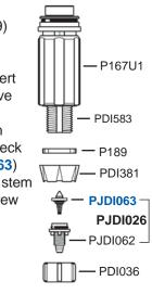
Pinch and remove the dosing seal and replace with the new one (Fig. 1) (JDI106).
