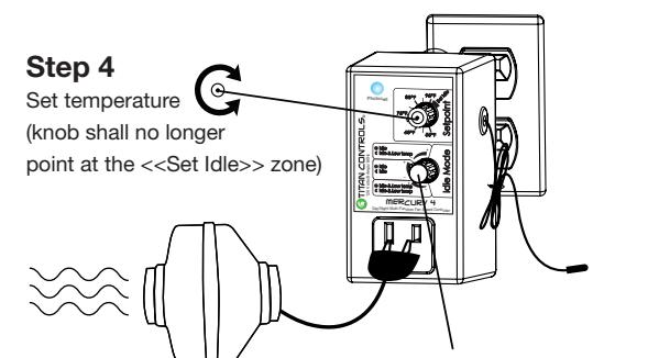
Bottom knob value is LATCHED when top knob leaves the <<Set Idle>> zone, therefore rotating bottom knob has no effect during normal operation.
