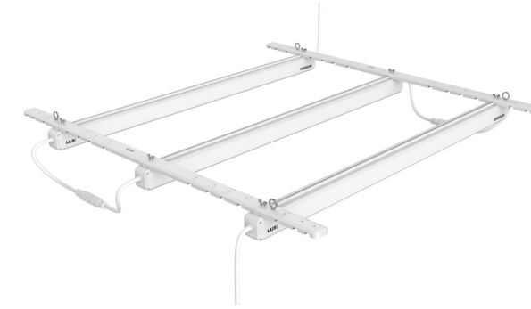
3 BAR | 600W | AVG PPFD: 537 5' FOOTPRINT | TESTED AT 24"
